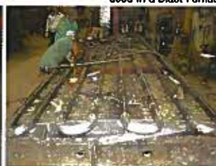
Coil manufacturing for a Cast Iron Stave used in a Blast Furnace
